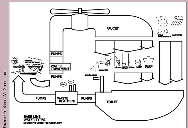
Figure 2 This simple illustration shows the municipal water treatment process as a large faucet that supplies high-quality water to a site. It also shows the typical municipal wastewater treatment system as a big toilet that carries away wastewater and treats it. The water from the faucet goes to several systems in a building. The plumbing engineer can design systems to reduce the size of the faucet and toilet.
