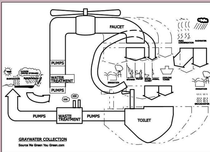
Figure 5 Installing graywater systems further reduces the size of the municipal faucet and toilet.
