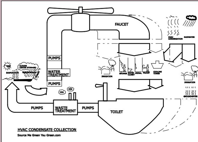
Figure 4 Collecting, treating, and distributing HVAC condensate to the building cooling tower system can reduce the size of the municipal faucet and toilet.
