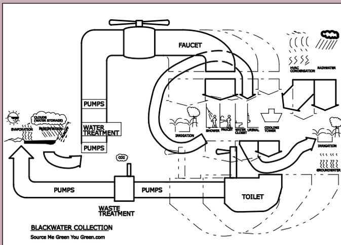
Figure 6 Black water systems can be expensive to install and operate safely, but when they are used, they can reduce flows in the municipal faucet and toilet.
