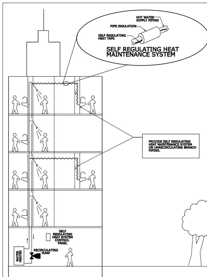
Figure 2 Self-regulating heat maintenance system on large building
