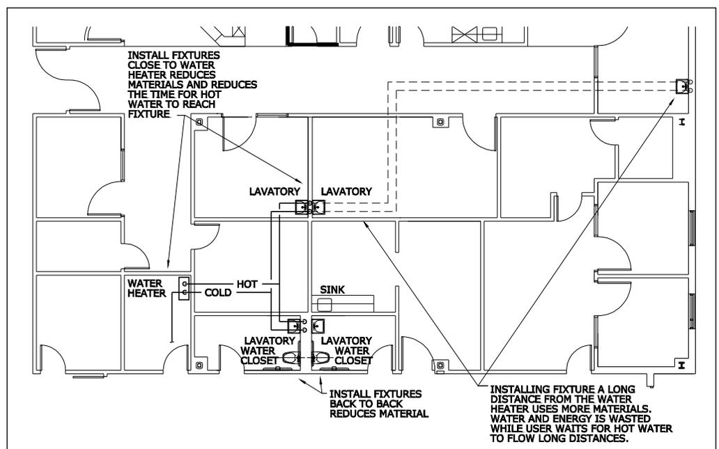
Figure 1 Floor plan with water piping layout
