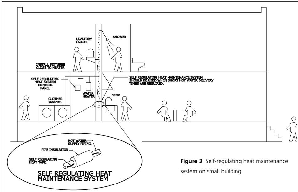
Figure 3 Self-regulating heat maintenance system on small building
